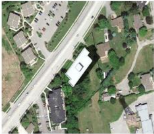
3:00 JUN 21 SHADING ENCROACHES ONTO ADJACENT PROPERTY TO THE EAST. MINOR SHADOWING ON THE WEST FACADE OF STRUCTURE.
