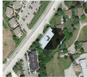
5:00 JUN 21 SHADING ENCROACHES ONTO ADJACENT PROPERTY TO THE EAST. SHADOWING ENCOUNTERED IMPACTS APPROXIMATELY 80% OF THE EXISTING RESIDENTIAL STRUCTURE AND REAR YARD.
