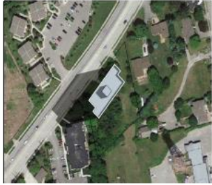
7:00 JUN 21 EARLY MORNING SHADOWING AFFECTS FRONT YARD OF PROPERTY TO WEST APARTMENT, AND PART OF THE ESSA ROAD RIGHT OF WAY. NO SIGNIFICANT IMPACT IS REALIZED.
