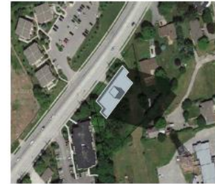
6:00 JUN 21 FULL SHADING OF ADJUTING RESIDENTIAL REAR YARD AND PARTIAL SHADING OF STRUCTURE IS ENCOUNTERED. MINOR SHADOWING PROJECTS ONTO REAR YARD OF RESIDENCE LOCATED AT 20 BEACON RD AS WELL AS THE NORTH-EAST CORNER OF THE RESIDENTIAL PROPERTY FRONTING ONTO SUNSET PL.
