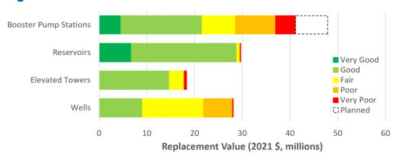
Figure 2-10 Condition of Vertical Facilities in the Ground Water System
